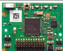
ZigBee-Pro Green Com-Funkplatine VCM8000V5094P
